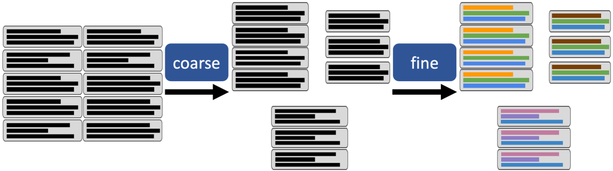
Figure 4.2: Pipeline for INFOSHIELD : Taking crawled ads as input, INFOSHIELD-coarse groups these ads into micro-clusters, and INFOSHIELD-fine highlights the common phrases in each ad by finding a common template.
