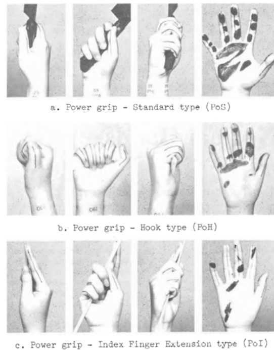
Figure 2.1: Early visualizations of human hand contact areas generated during various object grasps.
