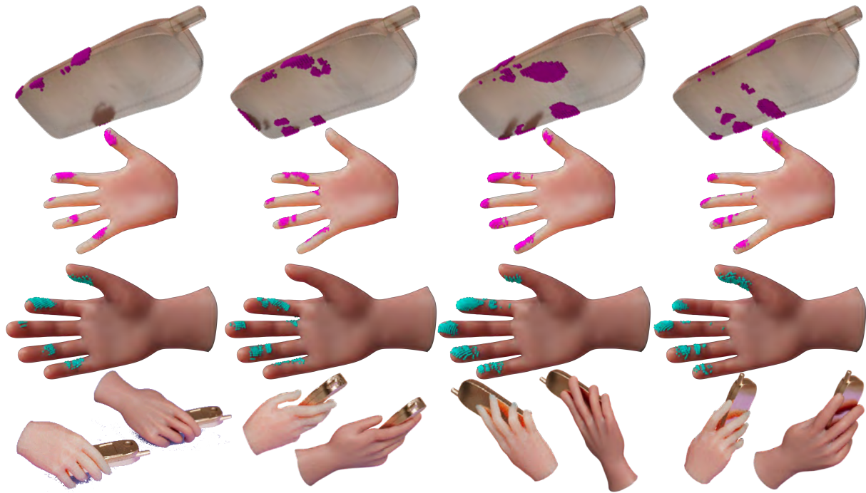
Figure 6.10: (Top Row) Object contacts, (Second Row) source hand contacts, (Third Row) computed target hand contacts, and (Bottom Row) source and retargeted hand motion for four different stages of a complex phone manipulation: (First Column) table pickup, (Second Column) in-hand dialing, (Third Column) holding for use, and (Last Column) movement back towards the table for release. Although poses and contact distributions vary dramatically during the manipulation, our method can successfully produce target hand motion by using source hand contact areas as a foundational retargeting medium.
