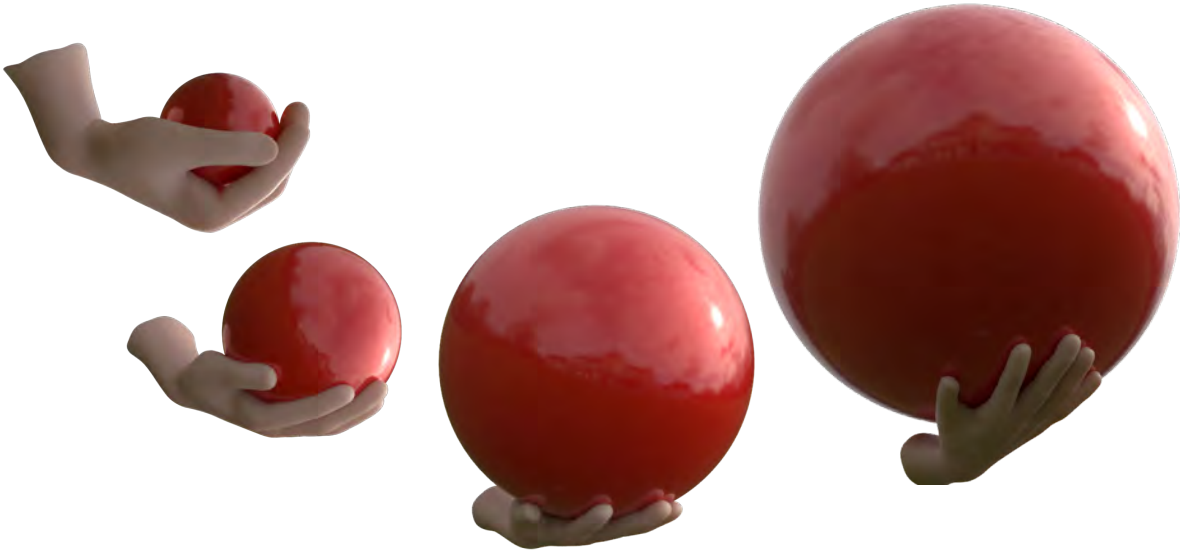
Figure 5.9: Demonstration of a manipulator adapting its grip in response to variance in object scale.
