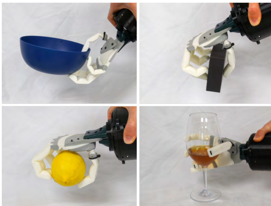
Figure 8.3: Based on the results in the design study shown in Figure 8.2 , candidate (d) is selected for fabrication. All grasps are successfully completed in a pick and place setup using key-framed open-loop poses that match the results obtained in our simulation.
