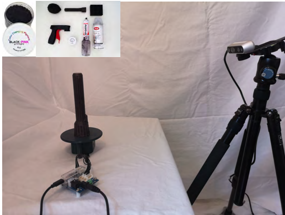
Figure 9.1: Capture setup used for thermochromic paint imaging along with (upper left) pigment and applicator materials.
