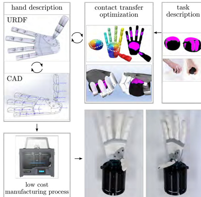
Figure 8.1: Iterative hand design prototyping framework enabled by contact area transfer and grasp computation
