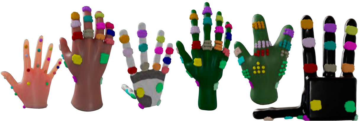
Figure 6.8: Single point virtual marker configuration on the source MANO hand and area based corresponding marker sets on all other hands. We use a manifold wrapper of the Allegro Hand for contact processing.
