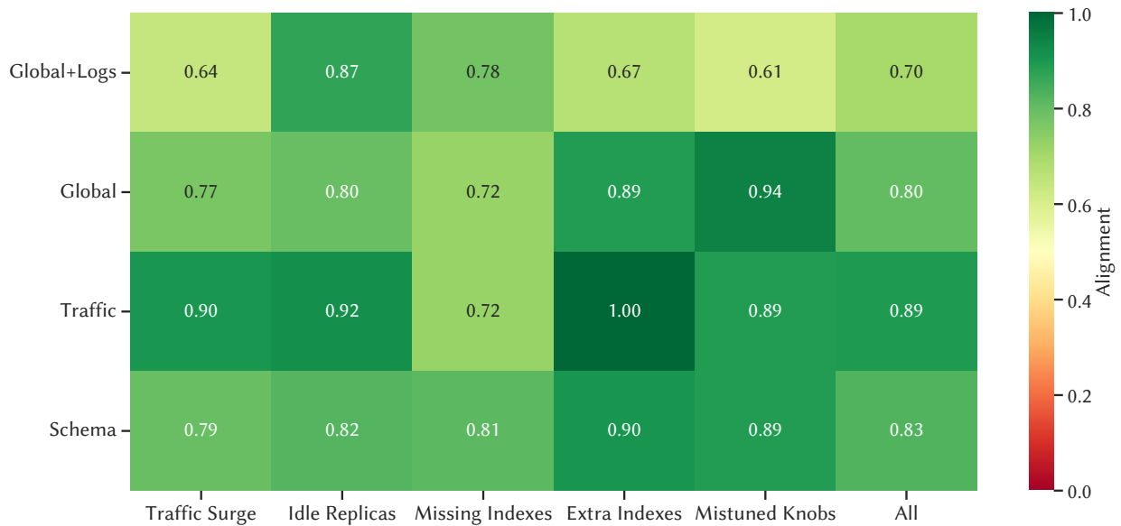
Figure 5.9: Tool-Hypothesis Alignment – Mean alignment score between hypotheses and subsequent optimization tool invocation across four contextual perspectives (Global+Logs, Global, Traffic, and Schema) and five scenarios (traffic surge, idle replicas, missing indexes, extra indexes, and mistuned knobs). Alignment scores are computed from a golden mapping from hypothesis category to tools.
