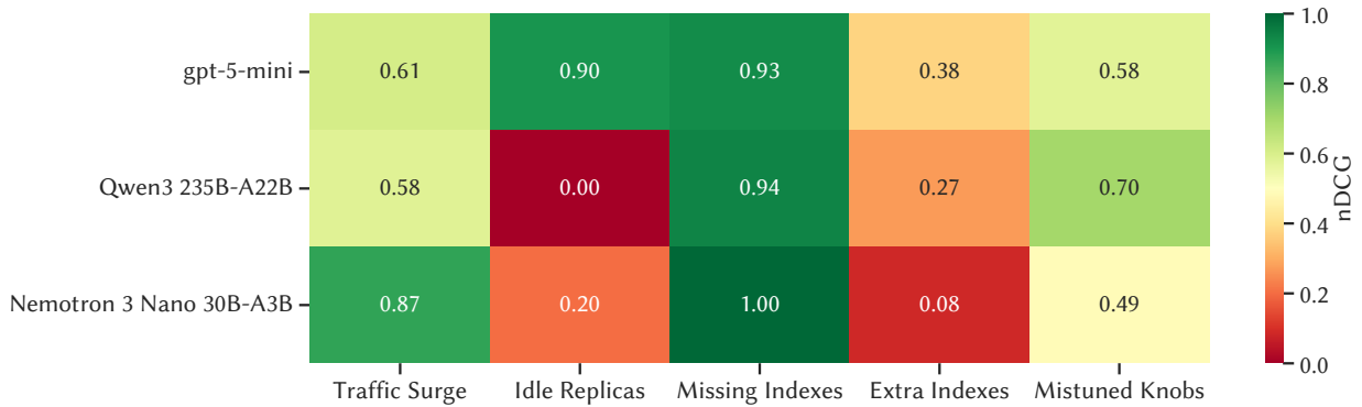
Figure 5.8: Reasoning Model – nDCG of ranked hypotheses generated from the Global+Logs context across five anomaly scenarios (traffic surge, idle replicas, missing indexes, extra indexes, and mistuned knobs). We evaluate three reasoning models of different sizes from largest to smallest: GPT-5-mini , Qwen3 235B-A22B , and Nemotron 3 Nano 30B-A3B .
